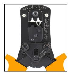
Open the tool, lay in the terminal and close the tool lightly until the terminal is held. Insert the cable.
